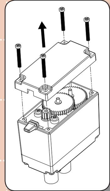
2. Remove the first cluster gear (as shown) and replace it with the Gear with the White/Black Encoder Wheel from the kit. Ensure the gear meshes with its two mating gears, and that the steel axles are still fully inserted into the plastic motor housing.
