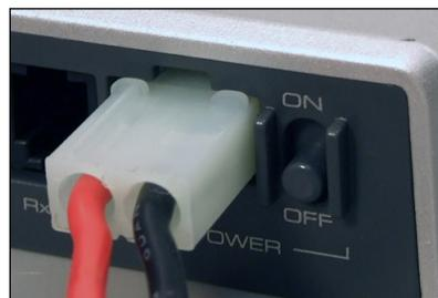
2. If you are programming over USB, connect the Cortex to the PC using the USB A-to-A cable. This will partially power the Cortex, then **turn the Cortex on** to fully power it using the battery.
