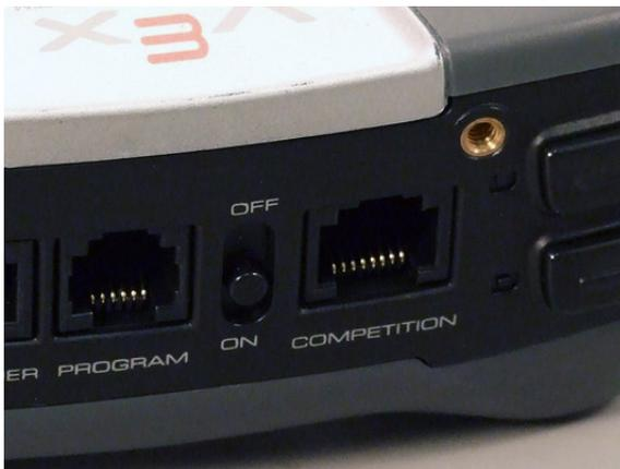
7b. Turn the VEXnet Remote Control ON
