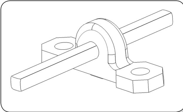
Another type of bearing used in the VEX Motion Subsystem is a Bearing Block; these are similar to the “pillow-blocks” used in industry. The Bearing Block mounts on a piece of structure and supports a shaft which is offset either above, below, or to the side of the structure.
