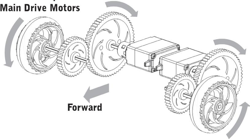
Use motors to power the robot's drive wheels. The wheels need to make continuous full rotations, which is exactly the kind of motion provided by the motors. Rotation for forward motion is shown.
