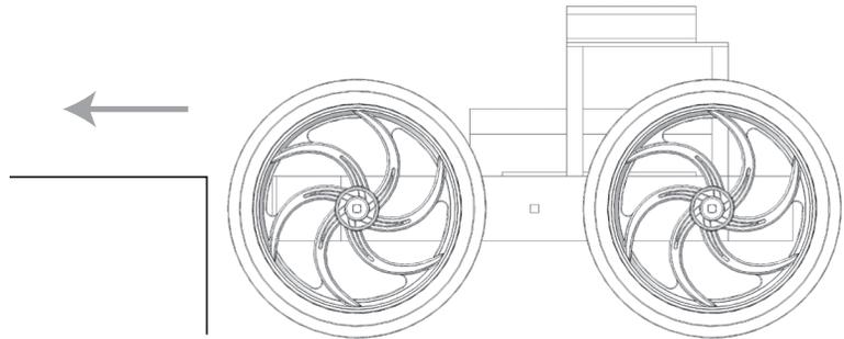
The robot with larger wheels has a much less difficult angle to climb to get up the step. This robot is much more likely to succeed.
