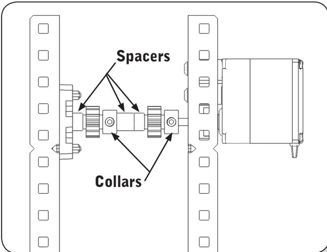
The Motion Subsystem also contains parts designed to keep pieces positioned on a VEX shaft. These pieces include washers, spacers, and shaft collars. VEX Shaft Collars slide onto a shaft, and can be fastened in place using a setscrew. Before tightening the setscrew, it is important to slide the Shaft Collars along the square shafts until they are next to a fixed part of the robot so that the collar prevents the shaft from sliding back and forth.
