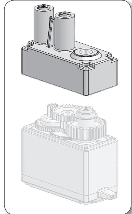
4. Remove the middle gear and the large shaft gear together.
