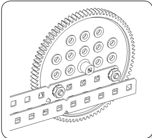
It is easy to drive components of the VEX Structure Subsystem using motion components in several different ways. Most of the VEX Gears have mounting holes in them on the standard VEX 1/2" hole spacing; it is simple to attach metal pieces to these mounting holes. One benefit of using this method is that in some configurations, the final gear train will transfer torque directly into the structural piece via a gear; this decreases the torque running through the shaft itself.
