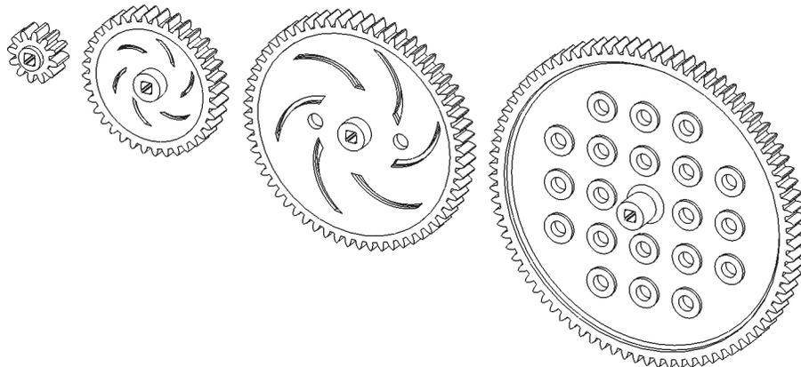
These gears can also be combined with sprocket & chain reductions, and also with advanced gear types to create even more complex mechanisms.
