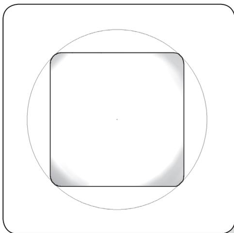
The square shaft has rounded corners which allow it to spin easily in a round hole. This allows the use of simple bearings made from Delrin (a slippery plastic). The Delrin bearing will provide a low-friction piece for the shafts to turn in.
