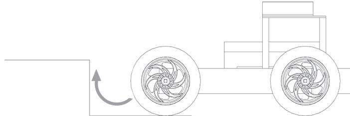
The robot with smaller wheels has a much steeper angle to climb – in fact, it's a sheer vertical face.
