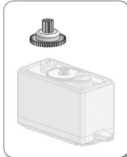
6. Remove the thin bottom gear, and carefully wipe the bottom gear deck and the inside of the top case to remove any remaining broken gear fragments.
