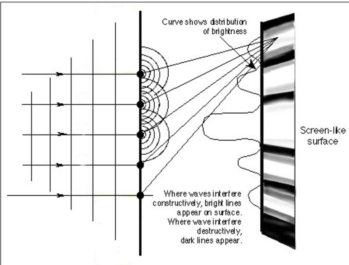
This diagram below shows how diffraction occurs through ‘slits’ (as opposed to the mesh ‘grids’ that are in the porthole). The general principles of diffraction and interference are the same in both cases.
