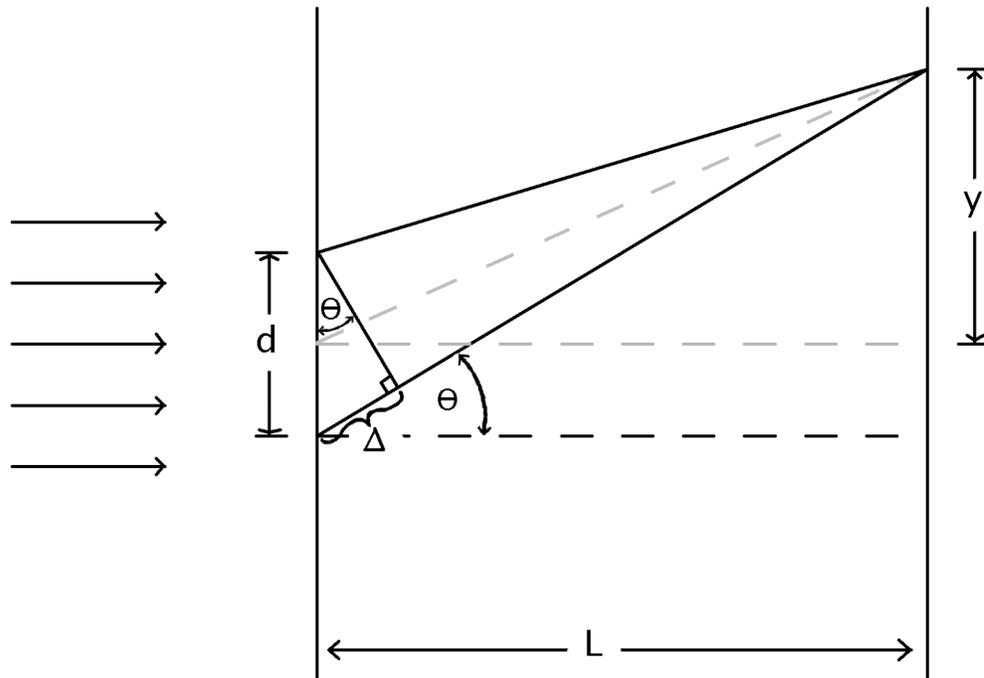
c. For  $L \gg d$ , you can use the above approximation of  $\theta$ . The beam (holes-to-spots) angle should be understood to be identical, by similarity, to the angle opposite  $\Delta$  and adjacent to  $d$ . Derive the Grating Equation  $n\lambda = d \sin \theta = \Delta$  either using trigonometry or “small angle approximation” where  $\sin \theta \sim \theta$  in radians  $\sim y/L$ . (Hint: Determine the ratio of the corresponding sides of two similar triangles.)
