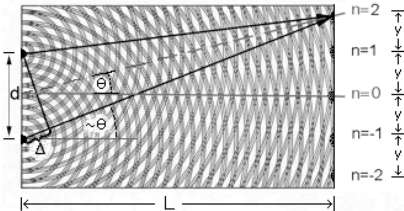
1. In the diagram above, a plane wave from the left hits these two holes separated by a spacing “ $d$ ”, and is diffracted to the right. A dashed line marks the path toward the  $n=2$  spot, which is at an angle  $\theta$  away from the central spot. The spots on the screen are separated by a spacing “ $y$ ”. In this picture, the rings show the peak of the waves, and the separation of the rings is the wavelength  $\lambda$ .
