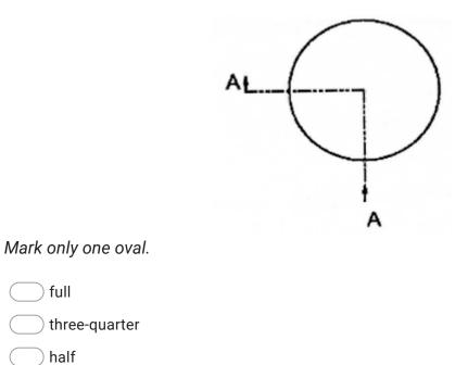
18. Which of the cutting plane lines shown below would indicate a 1/2 section? \*
